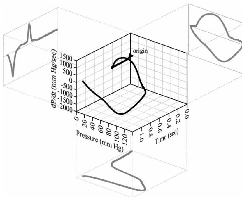
Fig. 2. Three-dimensional contour of time (*x*-axis) vs. pressure (*y*-axis) vs.  $dP/dt$  (*z*-axis; center, black plot) and 2-dimensional projections of the contour onto the phase plane ( $dP/dt$  vs. pressure), the pressure vs. time plane, and the  $dP/dt$  vs. time plane (gray plots, clockwise from top right).
