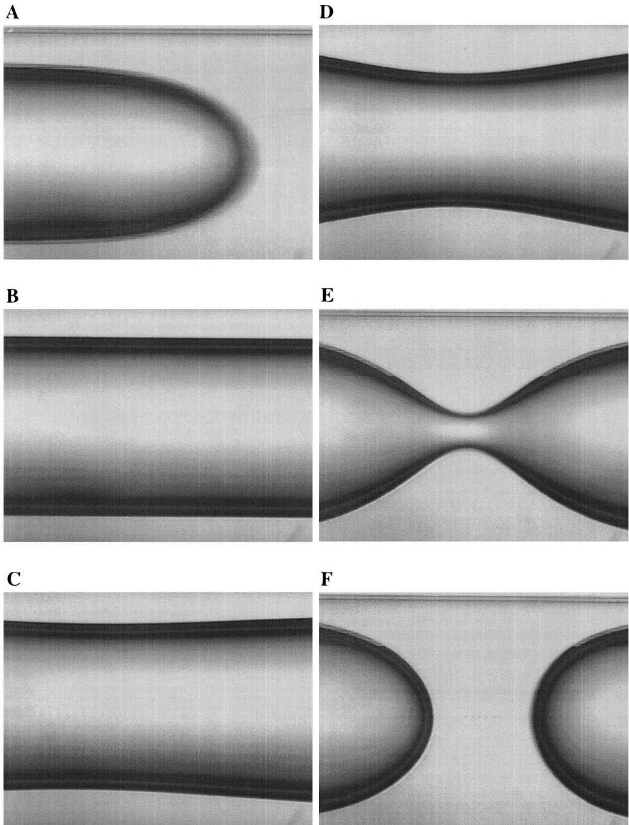
Fig. 3. Photographs of experimental procedure. Inflow begins (*A*) and a uniform film is established (*B*); then inflow is stopped, a small disturbance is located (*C*), and disturbance amplifies (*D*). *E*: just before closure. *F*: just after closure.
